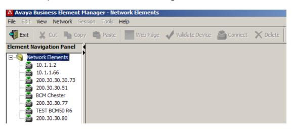
4. Open the **Network Elements** folder and select the IP Address of the BCM.
